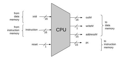
/\*\* The Hack Central Processing Unit consists of an ALU, two registers named A and D, and a program counter named PC (these internal chip-parts are not shown in the diagram). The inM input and outM output hold the values referred to as "M" in the Hack instruction syntax. The addressM output holds the memory address to which outM should be written.
