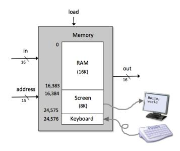
/\*\* The complete address space of the Hack computer's data memory, including RAM and memorymapped I/O. Facilitates read and write operations, as follows:
